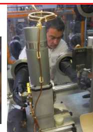
Glove box welding (LEFCA)
