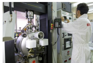
Thermomechanical characterisation (LBF) PROTEE (LEFCA)
