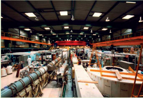
Fig. 14. The experimental hall of the Orphée reactor with its neutron guides in the foreground.
