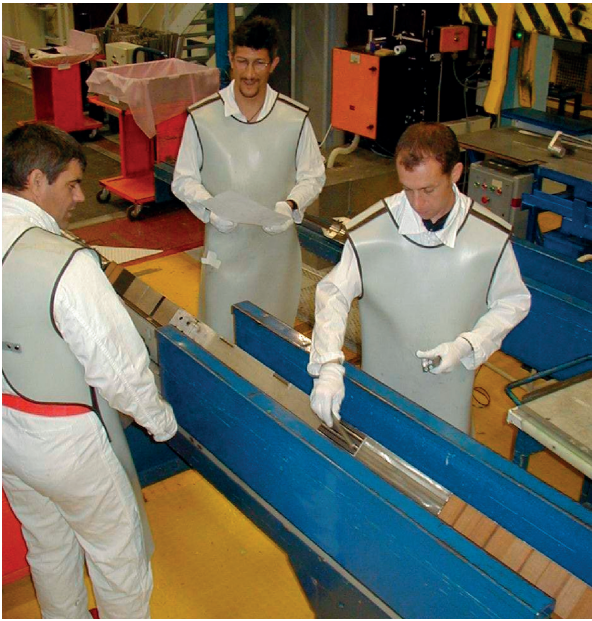
Fig. 51. Mounting of one of MASURCA assemblies in the Storage and Handling Building.
