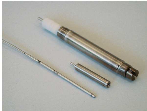
Fig. 42. Fission chambers for measuring neutron flux in the ÉOLE critical mockup.
