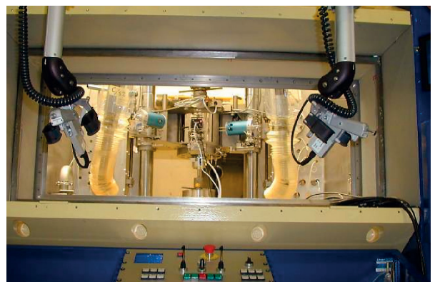
Fig. 79. A pulling machine in a LECI hot cell.
